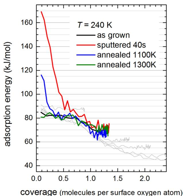
**Fig. 6** Adsorption energy of  $D_2O$  on the CaO(001) surface for sputter-induced surface defects based on deconvolution analysis using the initial 50 ms of the pulse time. The CaO(001) unit cell is defined as the number of surface O atoms ( $8.6 \times 10^{14}$  atoms per  $cm^2$ ). Each data point corresponds to an individual molecule pulse (connecting lines for better visibility)
