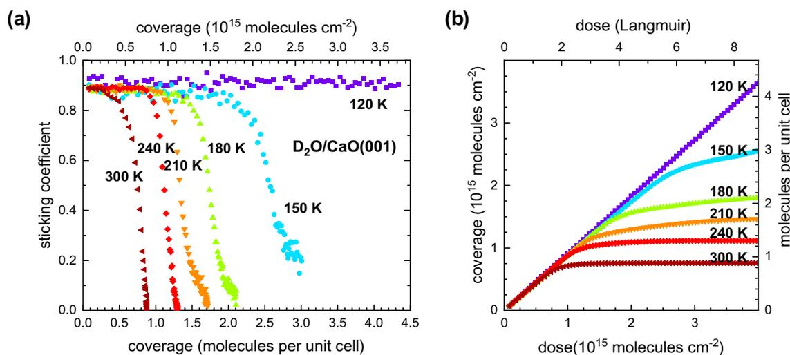
**Fig. 4** **a** Sticking coefficient for water adsorption on the CaO(001) surface and **b** resulting dependency of the surface coverage on the molecule dose for different surface temperatures. Each data point cor-
