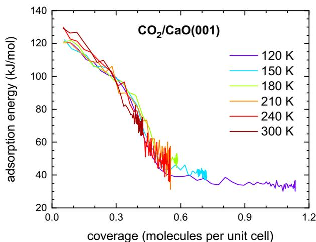
**Fig. 8** Adsorption energy from microcalorimetry for  $\text{CO}_2$  adsorption on the  $\text{CaO}(001)$  surface incorporating deconvolution of calorimetry and QMS data (initial 50 ms of pulse time). The  $\text{CaO}(001)$  unit cell is defined as the number of surface O atoms ( $8.6 \times 10^{14}$  atoms per  $\text{cm}^2$ ). Each data point corresponds to an individual molecule pulse (connecting lines for better visibility)
