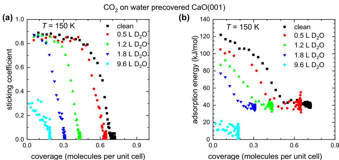
**Fig. 9** Sticking coefficient (a) and adsorption energy (b) for carbon dioxide adsorption on water covered CaO(001) surface after the indicated water dosages. The adsorption energy is based on deconvolu-
