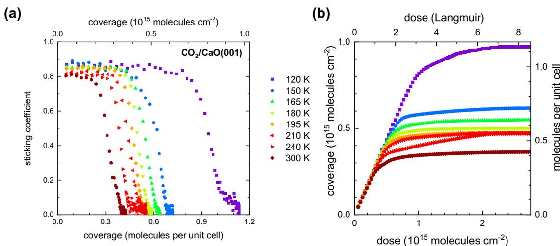
**Fig. 7** **a** Sticking coefficient for  $\text{CO}_2$  adsorption on  $\text{CaO}(001)$  and **b** resulting dependency of the surface coverage on the molecule dose for different surface temperatures. The  $\text{CaO}(001)$  unit cell is defined as the number of surface O atoms ( $8.6 \times 10^{14}$  atoms per  $\text{cm}^2$ )
