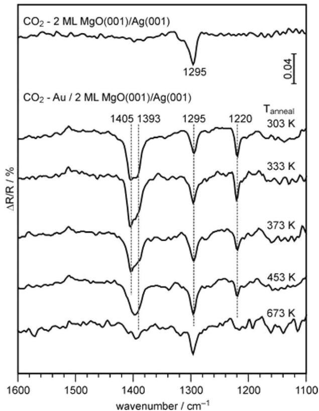
**Fig. 9** IRA spectra of bare (*top*) and Au-loaded 2 ML  $\text{MgO}(001)/\text{Ag}(001)$  samples recorded after a saturation dose of  $\text{CO}_2$  at 223 K. Au was deposited at 100 K and the samples subsequently annealed to the indicated temperature prior to  $\text{CO}_2$  adsorption (O'Brian et al. 2015)
