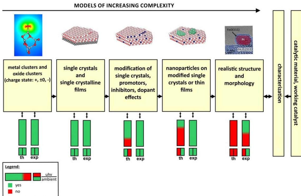
**Fig. 1** Schematic and pictorial representation of model systems as a function of increasing complexity to capture the essential features of a working catalyst. Each level is evaluated with respect to experiment and theory and with respect to progress that has been made to achieve
