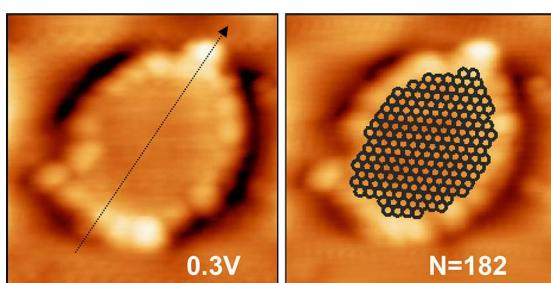
**Fig. 8** STM topological images of an Au particle with isophorone molecules at the rim (*left panel*), the Au island is schematically shown as a model. The *right hand panels* show a similarly shaped Au particle (Stiehler et al. 2015; Calaza et al. 2015)
