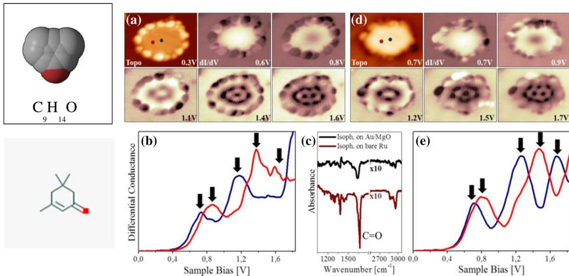
**Fig. 5** Topographic and  $dI/dV$  maps of an Au island (**a**) with and (**d**) without isophorone molecules (*left panels*) bound to its perimeter ( $11 \times 8 \text{ nm}^2$ ,  $70 \text{ pA}$ ). **b** and **e** associated conductance spectra taken in the center (blue) and the left part of the island (red) as indicated in (**a**) and (**d**). Gaussian fitting revealed five QWSs that are marked by
