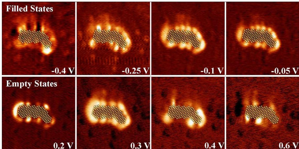
**Fig. 3** Filled and empty state  $dI/dV$  maps of the Au island shown in Fig. 1b. High  $dI/dV$  intensity is only observed along the island edges while the center remains *dark* at all bias voltages. An atomic model of the island is overlaid (Lin et al. 2010a)
