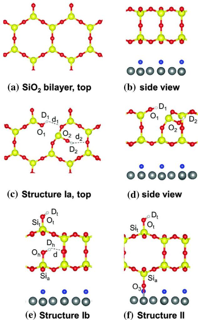
**Fig. 15** *Top* (a) and *side* (b) views of the pristine silica bilayer. *Top* (c) and *side* (d) views of the hydroxylation structure Ia. e *Side* view of the hydroxylated structure Ib. f *Side* view of the structure that forms a Si–O–Ru bridge to the Ru surface. Si, O and Ru atoms are shown in yellow, red, and gray, respectively. The O (or H for a H-precovered model,) atoms only adsorbed on the Ru(0001) surface are shown in blue (Yu et al. 2016) (color figure online)
