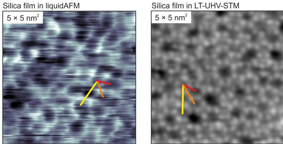
**Fig. 14** **a** Liquid-AFM image of an amorphous silica bilayer film show ring resolution ( $5 \times 5 \text{ nm}^2$ ,  $f = 337 \text{ kHz}$ ,  $A = 0.2 \text{ nm}$ ,  $k = 26.4 \text{ N/m}$ , 400 mM aqueous NaCl solution). **b** UHV-STM image of an amorphous silica bilayer film with atomic resolution of silicon atoms. ( $5 \times 5 \text{ nm}^2$ ,  $I_t = 50 \text{ pA}$ ,  $V_s = 2 \text{ V}$ ). The silicon atoms are
