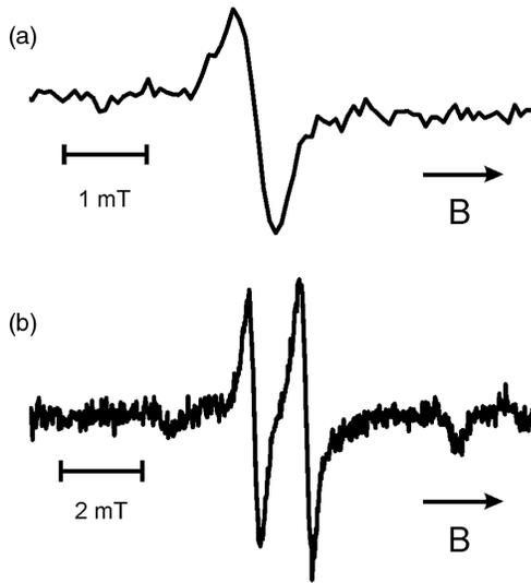
FIG. 1. EPR spectra of pristine MgO(001) films grown on Mo(001) at 300 K: (a) X-band EPR spectrum ( $T = 30$  K) of a 20-ML-thick film ( $\phi = 0^\circ$ ); (b) W-band EPR spectrum ( $T = 50$  K) of a 30-ML-thick film ( $\phi = 12^\circ$ ). The magnetic field is oriented in the surface plane.  $\phi$  denotes the angle between the magnetic field and a [110]-equivalent direction of the MgO lattice.
