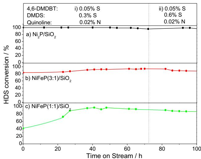
**Fig. 5.** Activity test at 340 °C in the HDS of 4,6-DMDBT for Ni<sub>2</sub>P/SiO<sub>2</sub>, NiFeP(3:1)/SiO<sub>2</sub> and NiFeP(1:1)/SiO<sub>2</sub>.
