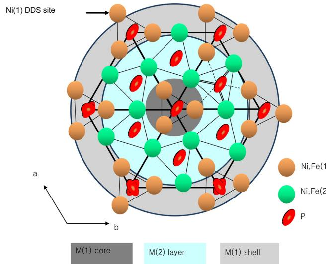
**Fig. 12.** Cross sectional schematic model of phosphide crystallites in Ni<sub>2</sub>P/SiO<sub>2</sub> and NiFeP(1:1)/SiO<sub>2</sub>.
