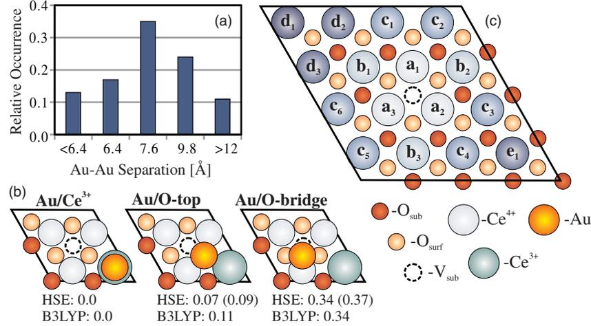
FIG. 3 (color online). (a) Distance histogram determined for  $\sim 150$  Au pairs on the ceria surface. (b) Relative energies [eV] obtained using HSE (optimized) and B3LYP (single point) for three relevant Au adsorption sites (Values in parenthesis include dispersion effects). (c)  $p(4 \times 4)$  unit cell with the notation of different Ce coordination shells around the  $V_{\text{sub}}$  defect, as used in Table I.
