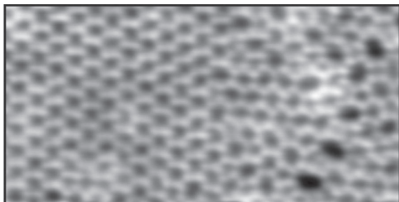
Figure 20. High resolution STM image (10 nm \times 5 nm) of a silica bilayer film, showing crystalline (left portion) and vitreous (right portion) phases coexisting.
