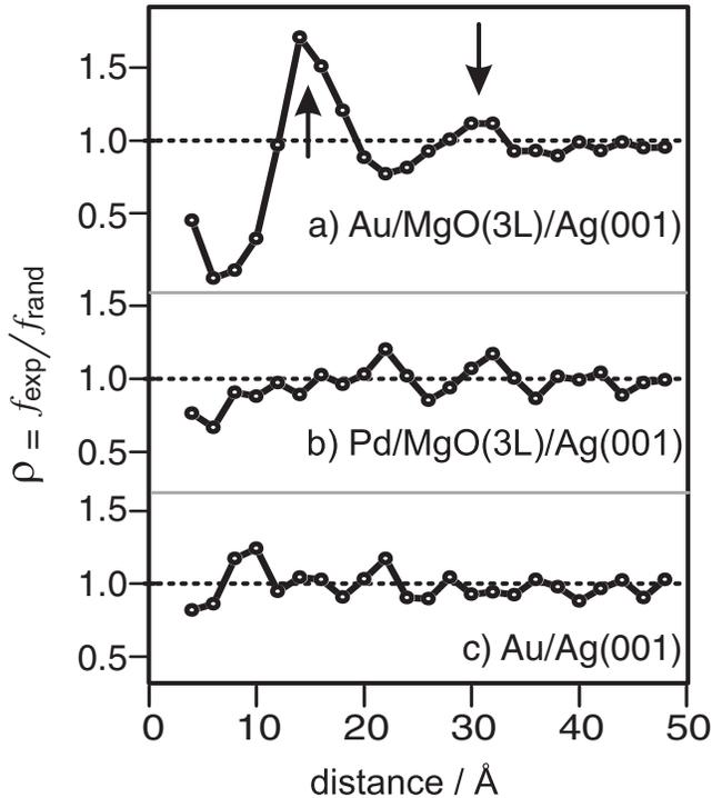
FIG. 2. Normalized radial pair distribution function  $\rho = f_{\text{exp}}(r)/f_{\text{rand}}(r)$  for pair distances up to  $r = 50$  Å for (a) Au atoms adsorbed on MgO(3L)/Ag(001), (b) Pd atoms adsorbed on MgO(3L)/Ag(001), and (c) Au atoms adsorbed on bare Ag(001).  $\rho = 1$  corresponds to random site occupation.
