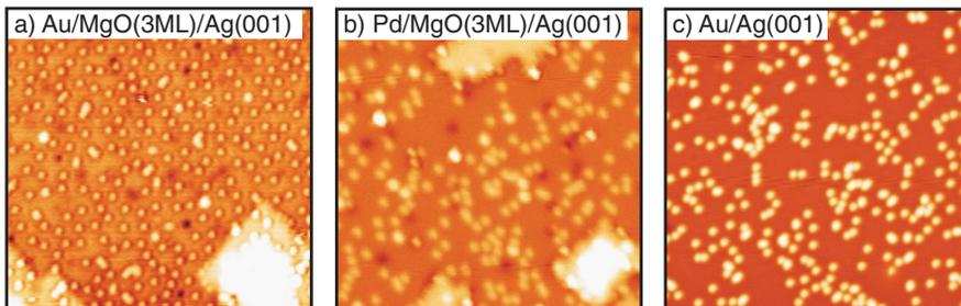
FIG. 1 (color online). STM images ( $30 \text{ nm} \times 30 \text{ nm}$ ) of (a) Au atoms adsorbed on 3 ML thin MgO films ( $\theta = 2.9\%$  ML Au,  $V_S = +0.5 \text{ V}$ ,  $I_T = 11 \text{ pA}$ ); (b) Pd atoms adsorbed on 3 ML thin MgO films ( $\theta = 2.3\%$  ML Pd,  $V_S = +0.2 \text{ V}$ ,  $I_T = 13 \text{ pA}$ ); (c) Au atoms adsorbed on bare Ag(001) ( $\theta = 2.9\%$  ML Au,  $V_S = +0.1 \text{ V}$ ,  $I_T = 100 \text{ pA}$ ).
