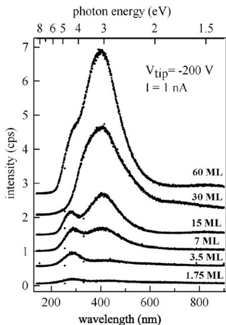
Fig. 3. Photon emission spectra collected from MgO films with increasing thickness. Excitation conditions were kept constant in all spectra (electron energy:  $-200$  eV, current:  $1$  nA, acquisition time:  $60$  s).
