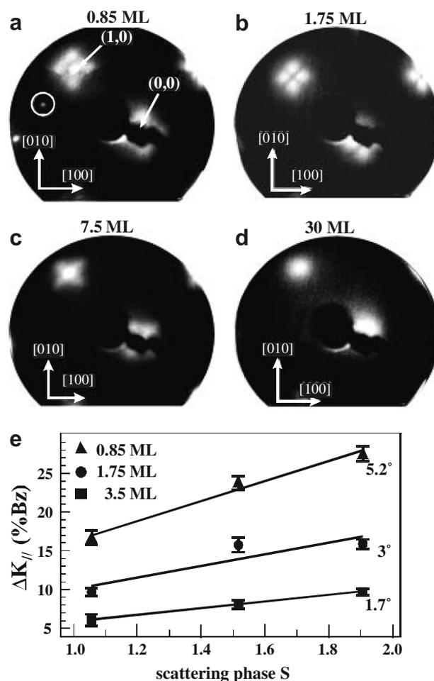
Fig. 1. LEED pattern of MgO films on Mo(001): (a) 0.85 ML, (b) 1.75 ML, (c) 7 ML and (d) 30 ML ( $E_p = 55$  eV). The circle in (a) marks one of the  $(2 \times 2)$  superstructure spots. (e) Positions of [100] satellites with respect to the central spot in the Brillouin zone shown as a function of the scattering phase  $S = dK_{\perp}/2\pi$  [21]. The lines are linear fits to the data and yield information on the tilting angles with respect to the ideal (001) surface.
