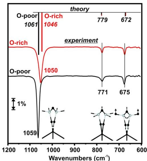
Fig. 4. IRAS spectra of the O-poor and O-rich silica films grown on  $\text{Mo}(112)$ . Calculated frequencies of the three IRAS most intense vibrations for 1 ML  $A$  and 1 ML  $A/4\text{O}$  structures are represented by the bars with the height proportional to the intensity normal to the surface.
