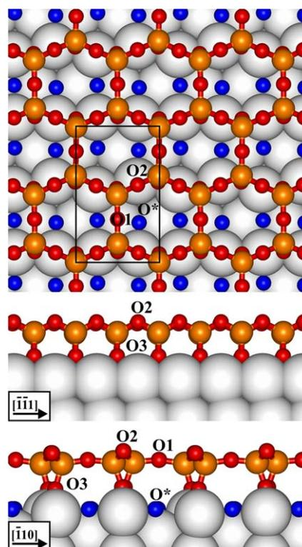
Fig. 2. Atomic structure of the O-rich (1 ML A/4O) phase of the 2D silica film on Mo(112). Oxygen atoms adsorbed on the Mo(112) surface ( $\text{O}^*$  species) are shown as blue spheres. The remaining O and Si atoms are represented by red and orange spheres, respectively. Surface unit cell is indicated as a black rectangle. (For interpretation of the references to colour in this figure legend, the reader is referred to the web version of this article.)
