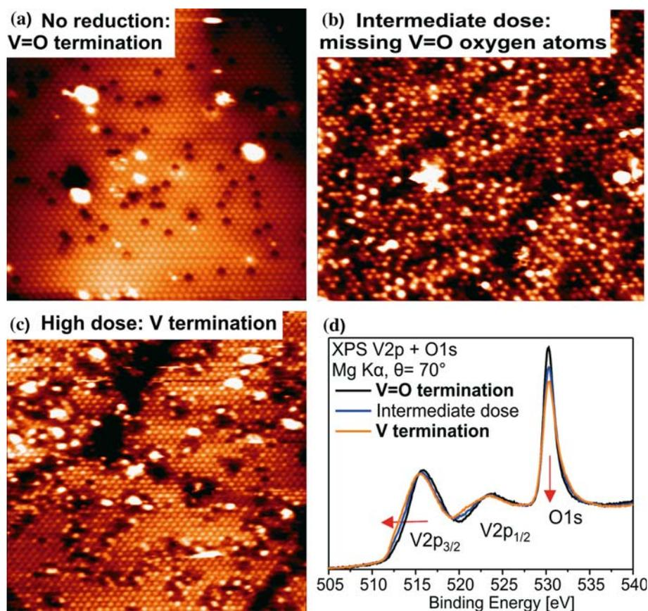
Figure 6. (a–c): STM images ( $20 \times 20$  nm,  $U = 2$  V,  $I = 0.2$  nA) of vanadyl-terminated (a), weakly reduced (b), and strongly reduced (c)  $\text{V}_2\text{O}_5(001)$  surfaces. Panel (d) shows corresponding XPS spectra.
