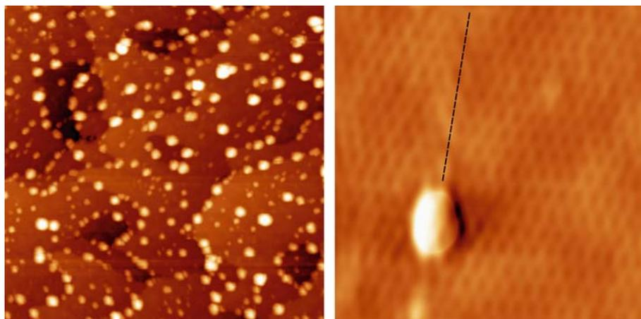
Figure 7. STM images of vanadia nanoparticles deposited on a model silica surface ( $\text{SiO}_2/\text{Mo}(112)$ ). Left image:  $100 \times 100$  nm,  $U = 3$  V,  $I = 0.2$  nA. Right image:  $10 \times 10$  nm,  $U = 1.5$  V,  $I = 0.2$  nA.
