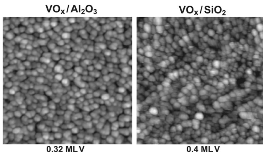
Figure 8. STM images ( $50 \times 50$  nm) of vanadia nanoparticles grown on a model alumina ( $\text{Al}_{10}\text{O}_{13}/\text{NiAl}(110)$ ) and a model silica ( $\text{Si}_4\text{O}_{10}/\text{Mo}(112)$ ) thin film. Left image:  $U = 2.2$  V,  $I = 0.07$  nA. Right image:  $U = 3.3$  V,  $I = 0.12$  nA.
