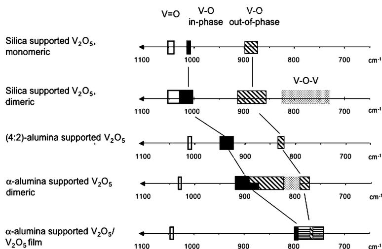
Figure 11. Wavenumber ranges for V=O (vanadyl) and V–O(–M) interphase modes for different vanadium oxide species and different supporting oxides. Data from Ref. [11], for  $\alpha$ -alumina supported dimeric  $\text{V}_2\text{O}_5$  from Ref. [9] and for  $\alpha$ -alumina supported  $\text{V}_2\text{O}_5$  film from Ref. [7]. For the latter, in phase and out-of-phase V–O(–M) modes cannot be distinguished and the range of V–O(–2Al) vibrations is marked by horizontal stripes.
