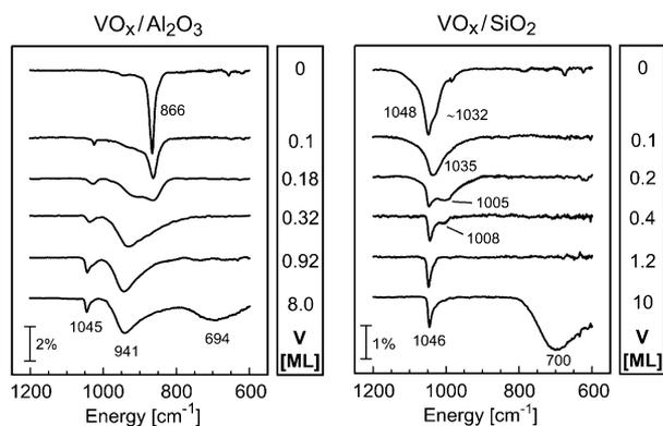
Figure 9. FT-IRAS spectra of clean (top)  $\text{Al}_{10}\text{O}_{13}/\text{NiAl}(110)$  (a) and  $\text{Si}_4\text{O}_{10}/\text{Mo}(112)$  (b) surfaces and after growing vanadia nanoparticles at different coverages given in monolayers (ML).
