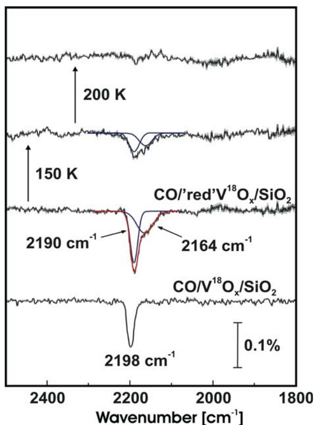
Figure 12. FT-IRAS spectra in the range of CO stretching frequencies for  $\text{VO}_x/\text{SiO}_2/\text{Mo}(112)$  exposed to CO. Non reduced system at the bottom in comparison with a reduced system at different temperatures.
