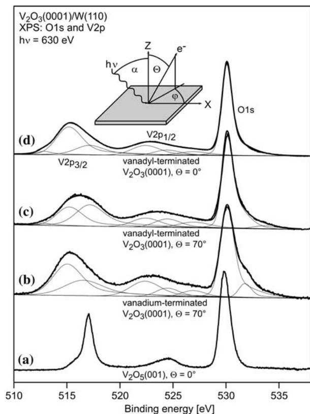
Figure 5. Photoelectron spectra of V<sub>2</sub>O<sub>3</sub>(0001) and V<sub>2</sub>O<sub>5</sub>(001) taken at different electron emission angles,  $\Theta$ .
