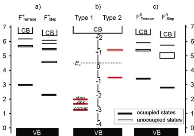
**Figure 4.** (a) Calculated energy levels of  $F^+$  centers on terrace and step sites. (b) Summary of energy levels of type 1 and type 2 defects from STM experiments. (c) Calculated energy levels of  $F^0$  centers on terrace and step sites.
