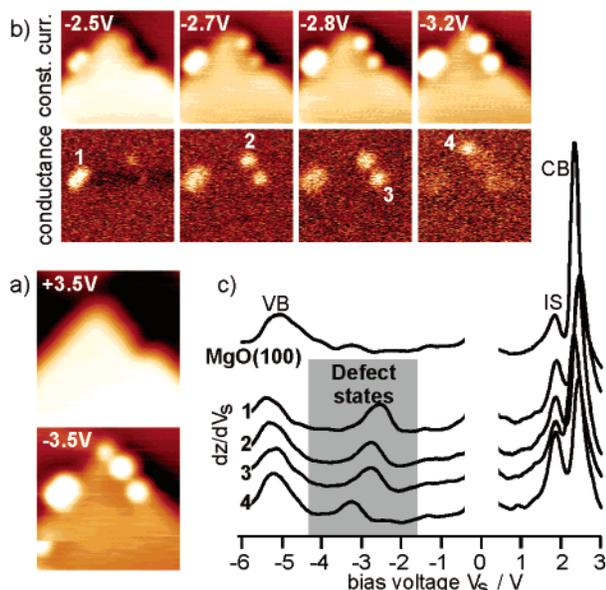
**Figure 2.** (a) STM images ( $5 \times 5 \text{ nm}^2$ ,  $I_t = 100 \text{ pA}$ ) of the morphology (at  $V_s = +3.5 \text{ V}$ ) and defect structure (at  $V_s = -3.5 \text{ V}$ ) of a MgO island on 4 ML MgO(001)/Ag(001). (b) Constant current and conductance images of defects located on the edges of a MgO island. (c)  $dz/dV_s$  spectra taken on the perfect MgO(001) island and at the defect locations.
