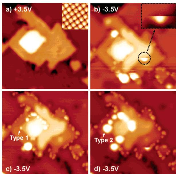
**Figure 1.** STM images ( $25 \times 25 \text{ nm}^2$ ,  $I_t = 100 \text{ pA}$ ) of a MgO island on 4 ML MgO(001)/Ag(001): (a)  $V_s = +3.5 \text{ V}$  (the inset shows the atomic resolution on a MgO terrace ( $15 \times 15 \text{ \AA}^2$ )); (b)  $V_s = -3.5 \text{ V}$  (the inset shows the magnification of the region, where a defect is changed during scanning); (c) and (d) images taken at  $V_s = -3.5 \text{ V}$ , after subsequent scanning at high positive bias voltages.
