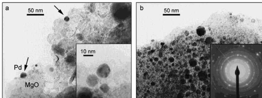
**Figure 2.** Transmission electron micrographs of Pd particles on polycrystalline MgO surfaces (2.5 wt % Pd): (a) Pd/MgO(Cl) (inset: particles with various shapes in higher magnification); (b) Pd/MgO(NO<sub>3</sub>) (inset: typical electron diffraction pattern; see text).
