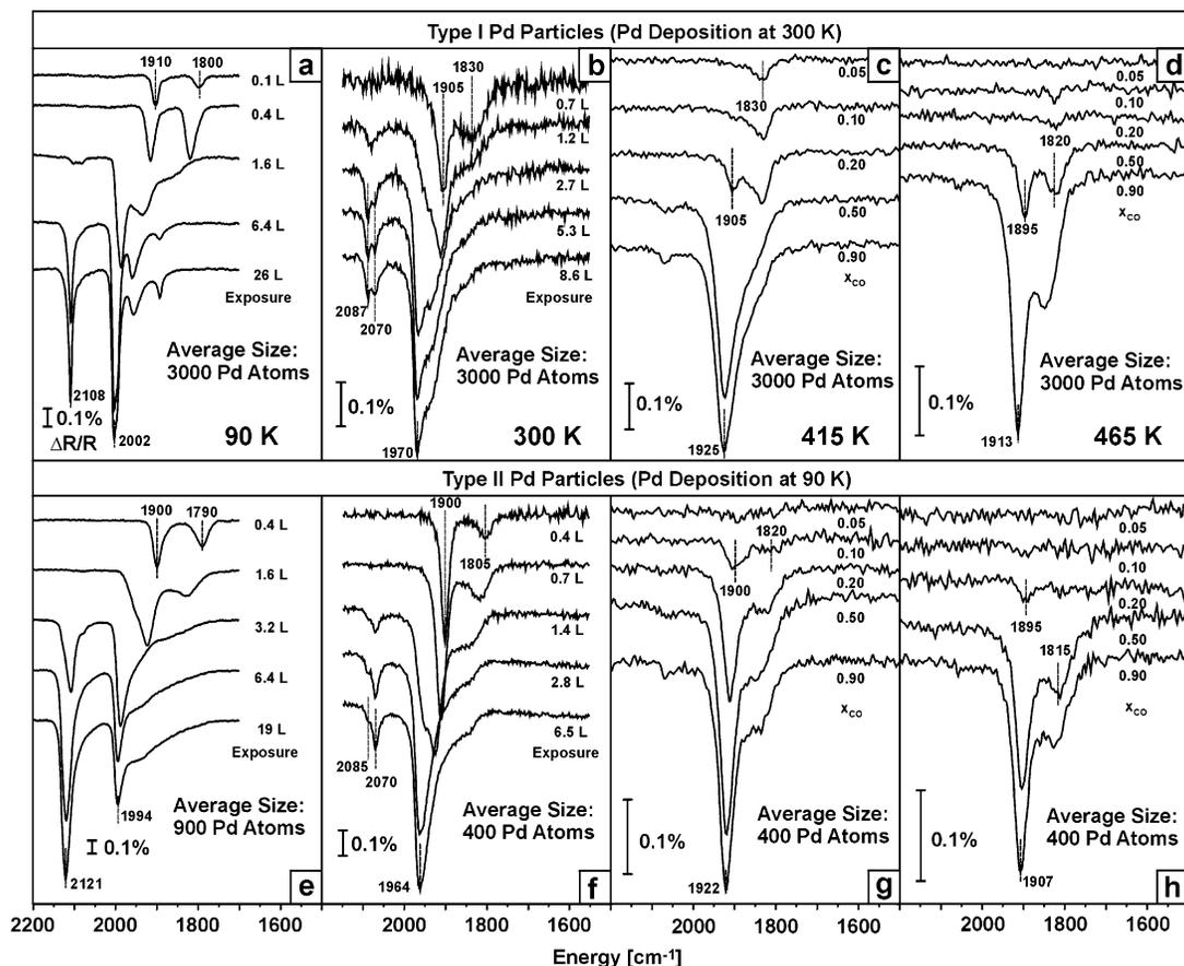
**Figure 8.** IR reflection absorption spectra for CO adsorbed on different Pd model catalysts: comparison of type I and type II particles and influence of the sample temperature and the CO coverage (see text for details).
