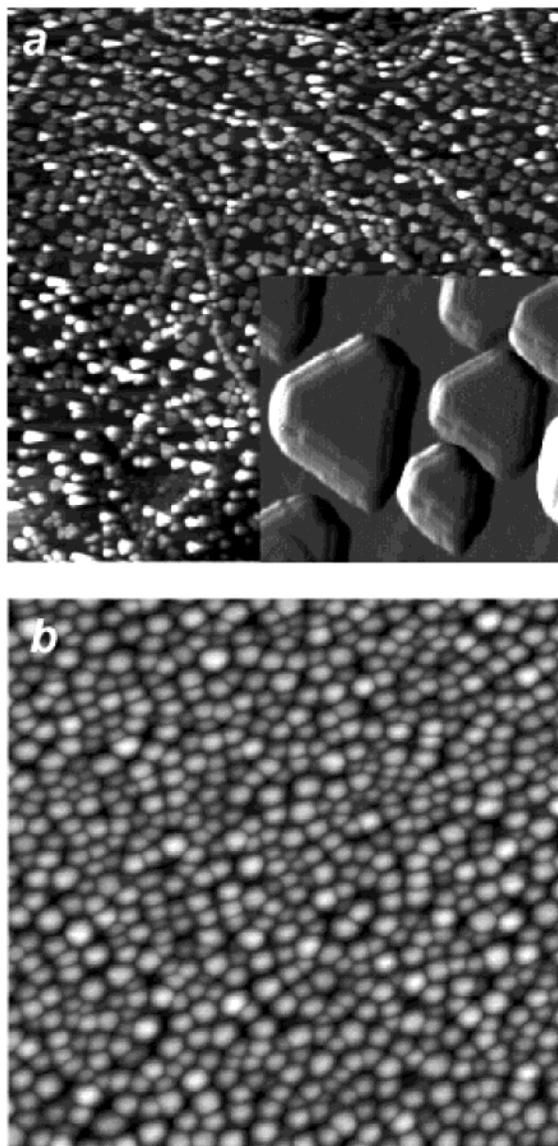
**Figure 3.** (a) Pd model catalyst of type I: STM image (3000 Å × 3000 Å) of Pd particles (approximately 3000 atoms/particle) grown at 300 K on Al<sub>2</sub>O<sub>3</sub>/NiAl(110). The inset shows a differentiated close-up STM image of the particles (200 Å × 200 Å).<sup>29</sup> (b) Pd model catalyst of type II: STM image (1000 Å × 1000 Å) of Pd particles (approximately 200 atoms/particle) grown at 90 K on Al<sub>2</sub>O<sub>3</sub>/NiAl(110) after heating to 500 K.<sup>32</sup>
