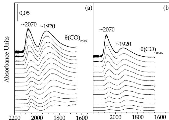
**Figure 4.** FTIR spectra in the CO stretching region from 2200 to 1500 cm<sup>-1</sup> of CO adsorbed at 300 K on Pd/γ-Al<sub>2</sub>O<sub>3</sub> (2.5 wt %) outgassed and reduced (a) at 623 K and (b) at 773 K ( $\theta_{\max}$ ,  $p(\text{CO}) = 2.66$  kPa;  $\theta_{\min}$ ,  $p(\text{CO}) \rightarrow 0$ ).
