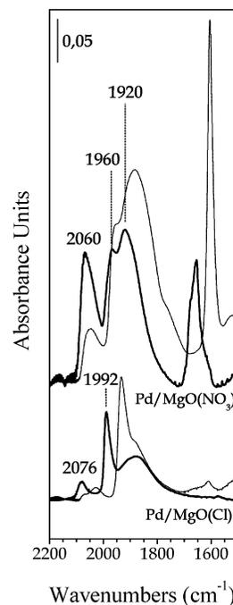
**Figure 10.** FTIR spectra in the CO stretching region from 2200 to 1500  $\text{cm}^{-1}$  of CO adsorbed at 300 K on Pd/MgO(Cl) (2.5 wt %) and Pd/MgO(NO<sub>3</sub>) samples outgassed and reduced at 623 K. Continuous curves refer to CO adsorbed on bare samples. Dotted curves refer to CO adsorbed on partially carbon covered samples (prepared by methanol decomposition; see text for details).
