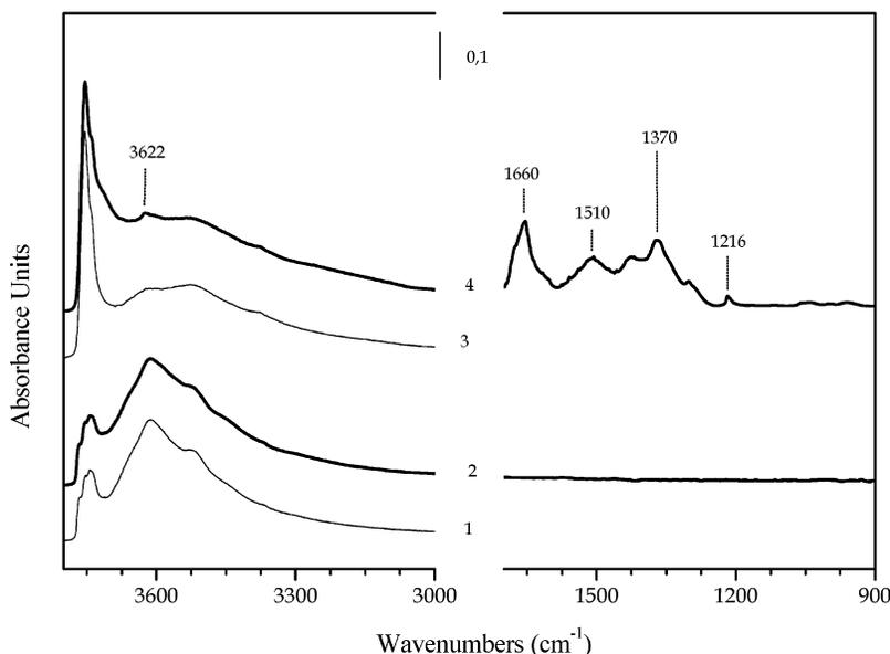
**Figure 6.** FTIR spectra in the 3800–3000 and 1700–900  $\text{cm}^{-1}$  ranges. Curves 1 and 3 show the spectra before CO adsorption on Pd/MgO(Cl) and Pd/MgO( $\text{NO}_3$ ), respectively; curves 2 and 4 show the spectra at  $\theta(\text{CO})_{\text{max}}$  ( $p = 2.66 \text{ kPa}$ ) on Pd/MgO(Cl) and Pd/MgO( $\text{NO}_3$ ), respectively.
