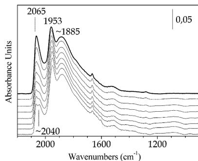
**Figure 7.** FTIR spectra in the CO stretching region from 2200 to 900  $\text{cm}^{-1}$  of CO adsorbed at 300 K on precovered hydrogen Pd/MgO( $\text{NO}_3$ ) outgassed and reduced at 673 K ( $\theta_{\text{max}}, p(\text{CO}) = 2.66 \text{ kPa}$ ;  $\theta_{\text{min}}, p(\text{CO}) \rightarrow 0$ ).
