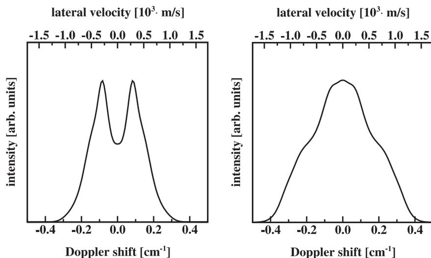
**FIGURE 6** Theoretical Doppler profiles and lateral velocity distributions, respectively, of CO molecules desorbing from Cr<sub>2</sub>O<sub>3</sub>(0001) within the states  $j'' = 12$  (left profile) and  $j'' = 31$  (right profile) integrated over all desorption velocities
