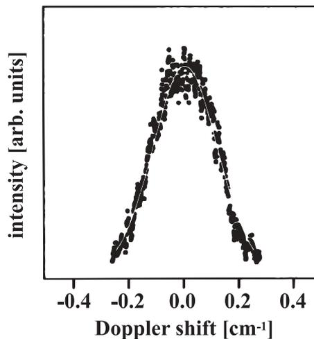
**FIGURE 4** Experimental Doppler profiles of CO molecules desorbing from Cr<sub>2</sub>O<sub>3</sub>(0001) within the states  $v'' = 0, j'' = 8$  (left profile) and  $v'' = 0, j'' = 31$  (right profile) for the desorption velocity  $1160 \text{ m s}^{-1}$ . The fitted curves indicated by solid white lines result from (6)
