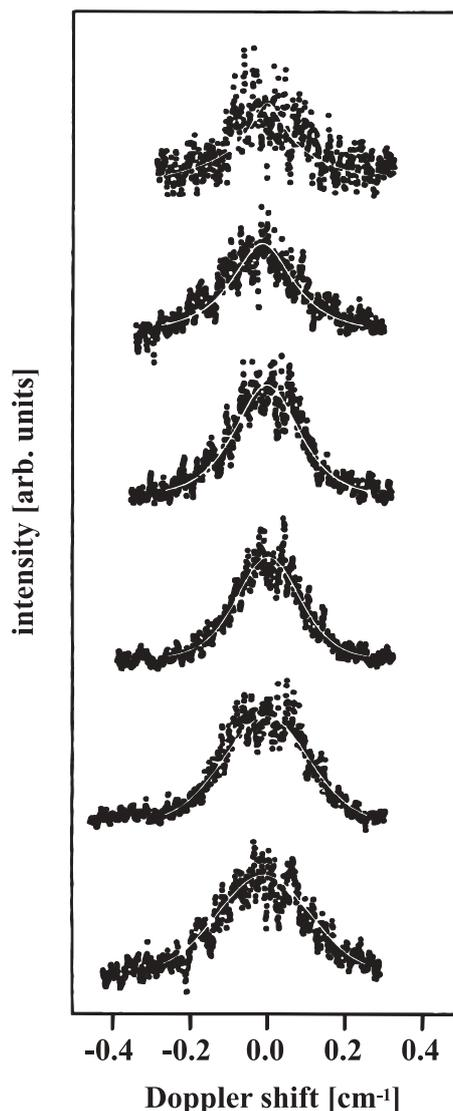
**FIGURE 3** Experimental Doppler profiles of CO molecules desorbing from Cr<sub>2</sub>O<sub>3</sub>(0001) within the state  $v'' = 0, j'' = 12$  for several desorption velocities:  $145 \text{ m s}^{-1}$  (topmost profile),  $340 \text{ m s}^{-1}$ ,  $480 \text{ m s}^{-1}$ ,  $650 \text{ m s}^{-1}$ ,  $1160 \text{ m s}^{-1}$  and  $1930 \text{ m s}^{-1}$  (lowest profile). The fitted curves indicated by solid white lines result from (6)
