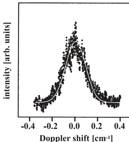
**FIGURE 2** Experimental Doppler profile of CO molecules in gas phase within the state  $v'' = 0$ ,  $j'' = 7$  at 303 K. The curve indicated by the solid white line results from kinetic gas theory (equation (3))
