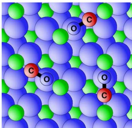
**FIGURE 1** Structure model for CO molecules adsorbed on a Cr<sub>2</sub>O<sub>3</sub>(0001) surface [22]
