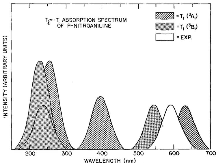
**Fig. 6.** A comparison of the experimental (Ref. [7]) and calculated  $T_1 \leftarrow T_1$  absorption spectra of PNA assuming a  $^3B_1$  and  $^3A_1$   $T_1$  character. The calculated spectra have been normalized separately so that the respective long wavelength excitation intensity corresponds with experiment
