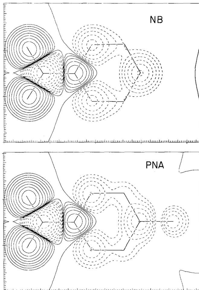
**Fig. 4.** Electron density difference diagrams for the NB and PNA  $1^3B_1(\pi^* \leftarrow n(\pi))$  excitation at  $1.5 \text{ \AA}$  above the molecular plane. Solid lines correspond to a positive charge density difference relative to  $S_0$ , whereas dashed lines represent a negative charge density difference
