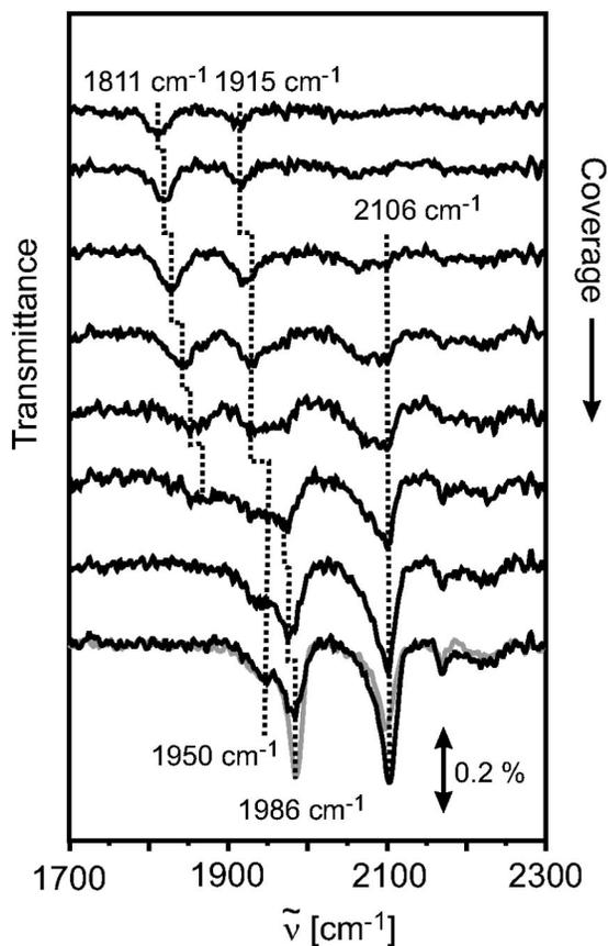
FIG. 5. IR spectra of adsorbed CO on 2 Å Pd particles with subsequently deposited 0.1 Å Co on the alumina film taken at 44 K as a function of CO coverage. The IR spectrum at saturation coverage of pure Pd (2 Å) is shown for comparison (gray trace) in the bottom panel.
