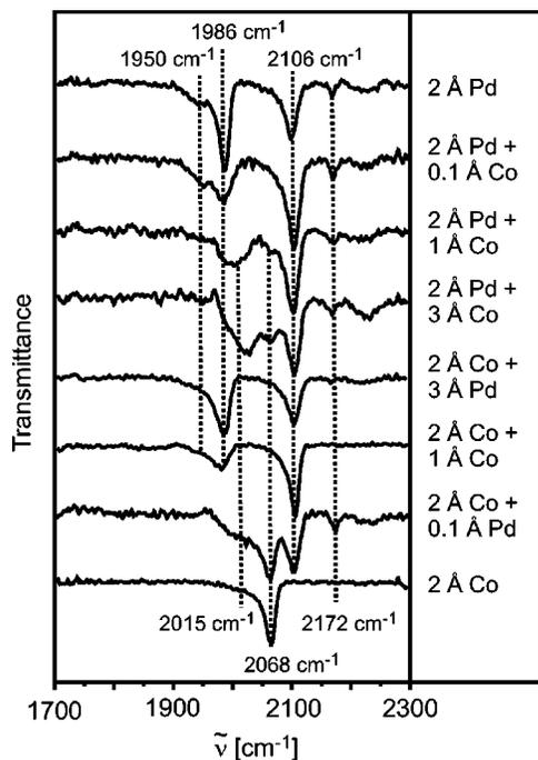
FIG. 9. IR spectra of CO adsorbed on various Co–Pd bimetallic particles supported on an alumina thin film. The designation 2 Å Co + 1 Å Pd designates a subsequent deposition of 2 Å Co and then 1 Å Pd at 300 K. Spectra were taken at 44 K.
