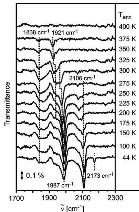
FIG. 4. IR spectra of adsorbed CO on 2 Å Co particles with subsequently deposited 1 Å Pd on the alumina film taken at 44 K as a function of temperature. The sample was exposed to CO at 44 K until saturated and then annealed to the various temperatures; all spectra were taken at 44 K.
