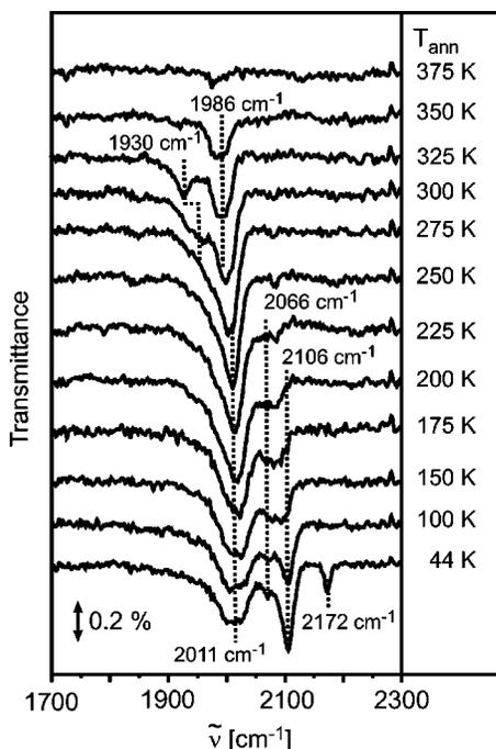
FIG. 7. IR spectra of adsorbed CO on 2 Å Pd particles with subsequently deposited 1 Å Co on the alumina film taken at 44 K as a function of temperature. The sample was exposed to CO at 44 K until saturated and then annealed to the various temperatures; all spectra were taken at 44 K.
