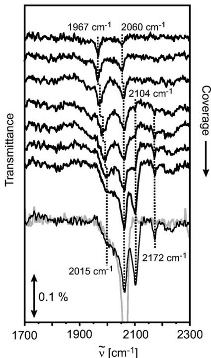
FIG. 2. IR spectra of adsorbed CO on 2 Å Co particles with subsequently deposited 0.1 Å Pd on the alumina film taken at 44 K as a function of CO coverage. The IR spectrum at saturation coverage of pure Co (2 Å) is shown for comparison (gray trace) in the bottom panel.
