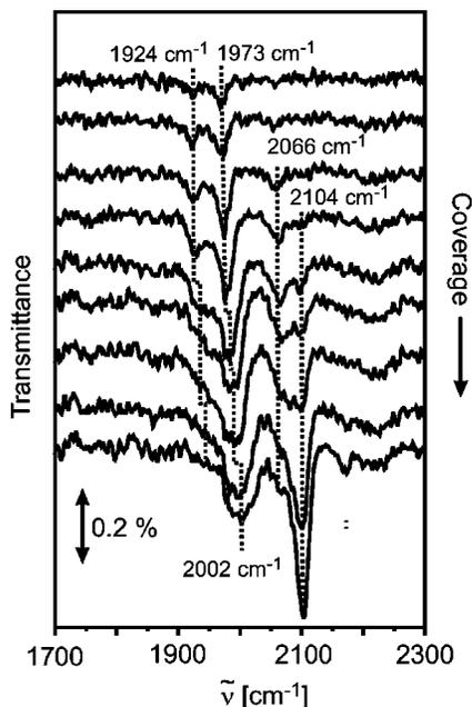
FIG. 6. IR spectra of adsorbed CO on 2 Å Pd particles with subsequently deposited 1 Å Co on the alumina film taken at 44 K as a function of CO coverage.
