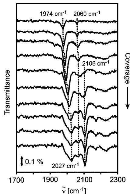
FIG. 8. IR spectra of adsorbed CO on 2 Å Pd particles with subsequently deposited 3 Å Co on the alumina film taken at 44 K as a function of CO coverage.
