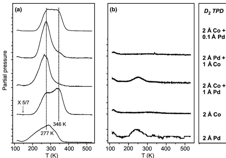
Fig. 2. TPD of D<sub>2</sub> from the pristine (a) and oxygen treated particles (b). All curves in part (b) are on the same partial pressure scale.
