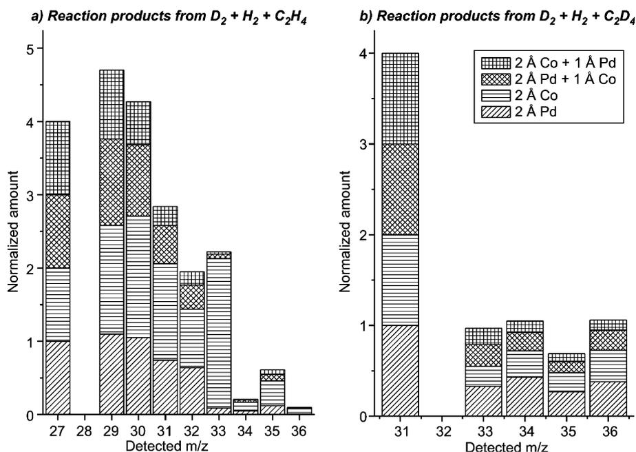
Fig. 4. Relative detected mass to charge ratios resulting from the reaction of  $D_2$  with  $C_2H_4$  and  $C_2D_4$ , respectively, on the bimetallic particles. The data were obtained in a multi-mass TPD experiment carried out in the temperature range from 100 to 500 K. In all cases, some  $H_2$  was present in the background.
