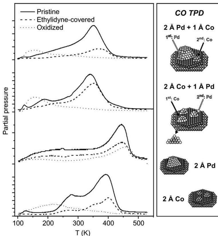
Fig. 1. TPD of CO from the pristine, ethylidyne-covered, and oxygen treated Co–Pd particles.
