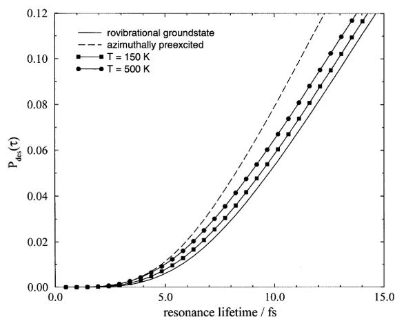
Fig. 7. Lifetime averaged desorption probabilities for different temperatures; the lifetime averaged desorption probability after selective excitation of an azimuthally preexcited state is shown for comparison (dashed line).
