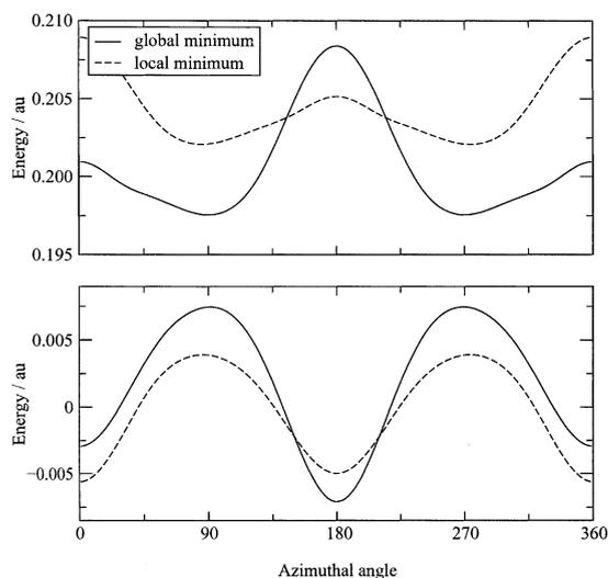
Fig. 6.  $\phi$ -Corrugation of electronic ground state (bottom) and electronically excited state (top). Straight line: situation at  $Z = 4.5$  a.u. and  $\theta = 122^\circ$  (global minimum). Dashed line: situation at  $Z = 4.9$  a.u. and  $\theta = 111^\circ$  (local minimum).
