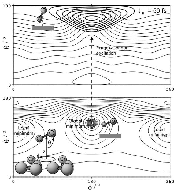
Fig. 1. 2D contour plots of the ab initio PES for the CO/Cr<sub>2</sub>O<sub>3</sub>(0 0 0 1)-system:  $\theta$ - $\phi$ -dependences at ground state equilibrium value for the CO-distance ( $Z = 4.5$  Bohr). Bottom: Electronic ground state with lowest rovibrational nuclear eigenstate. Top: Electronically excited  $a^3\Pi$ -state with snapshot of the wave packet after a time evolution of 50 fs. Inset: Cluster model used to represent the Cr<sub>2</sub>O<sub>3</sub>(0001)-surface.
