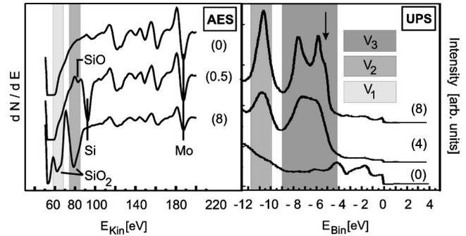
FIG. 6. *Left panel:* Differentiated AE spectra of the clean Mo(112) surface (0), clean Si on Mo(112) (0.5), and the silica film on the Mo(112) substrate (8). *Right panel:* He I UPS valence band study of the clean Mo(112) surface (0), the freshly deposited silica film (4) and the final silica epilayer on the Mo(112) surface (8). The gray panels  $V_1$ ,  $V_2$ , and  $V_3$  depict the contributions of the three well-known silica valence band regions to the spectra (see text).
