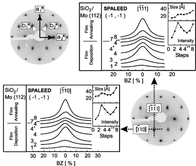
FIG. 2. SPA-LEED data ( $E = 56\text{ eV}$ ) of the  $(-1, -1)$  superlattice spot profiles along the  $[\bar{1}\bar{1}1]$  and the  $[\bar{1}10]$  direction during the silica film deposition ( $1-4^{++}$ ) and during the silica film annealing procedure ( $7$  and  $8$ ). Along each of these substrate directions, the size of the crystalline silica domains (upper insets) and the integrated profile intensity (lower insets) have been derived during the silica film preparation.
