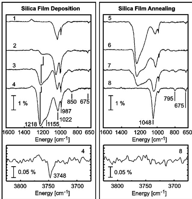
FIG. 5. IRAS spectra of the silica epilayer on the Mo(112) surface during the deposition (1–4) and the annealing (5–8) steps. The upper (bottom) panels show the spectral region from 650 to 1600  $\text{cm}^{-1}$  (3600 to 3900  $\text{cm}^{-1}$ ) (see text).
