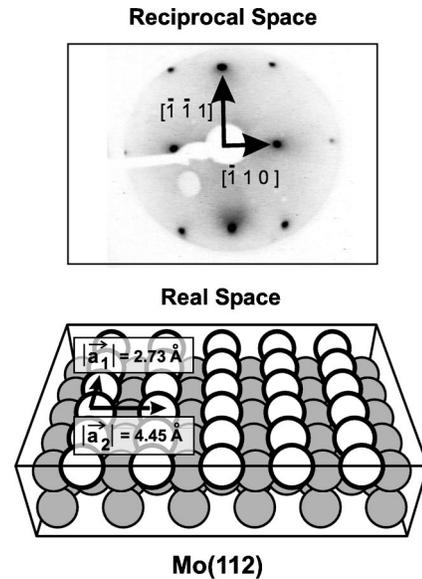
FIG. 1. LEED pattern ( $E = 56\text{ eV}$ ) and perspective view of the trough and row structure of the Mo(112) surface. The rectangular surface unit mesh is indicated in the reciprocal as well as in the real space image.
