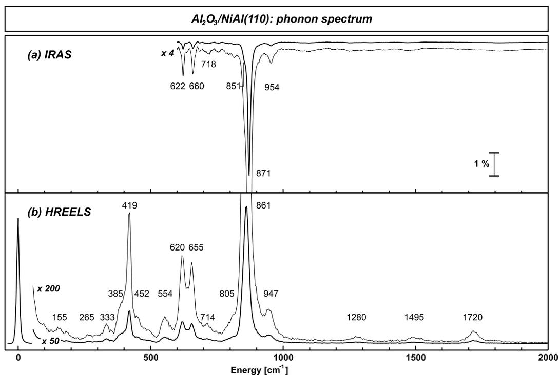
Fig. 2. (a) Infrared and (b) HREEL spectra of the alumina film recorded at 90 K.
