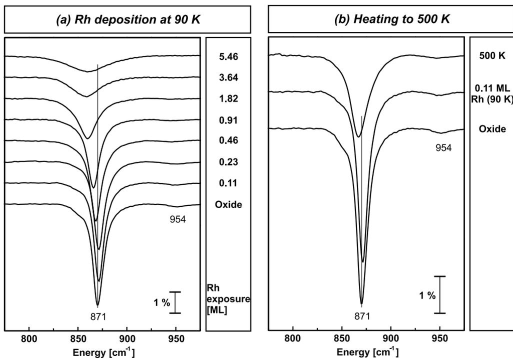
Fig. 4. (a) Infrared spectra of the alumina film in the region of its most intense phonon mode  $\nu_3$  for the clean film (bottom) and after exposing the film to increasing amounts of Rh at 90 K. (b) Infrared spectra of the alumina film in the region of its most intense phonon mode  $\nu_3$  for the clean film (bottom), after exposing the film to 0.11 ML Rh at 90 K (center) and after subsequent annealing to 500 K (top). All spectra were recorded at 90 K.
