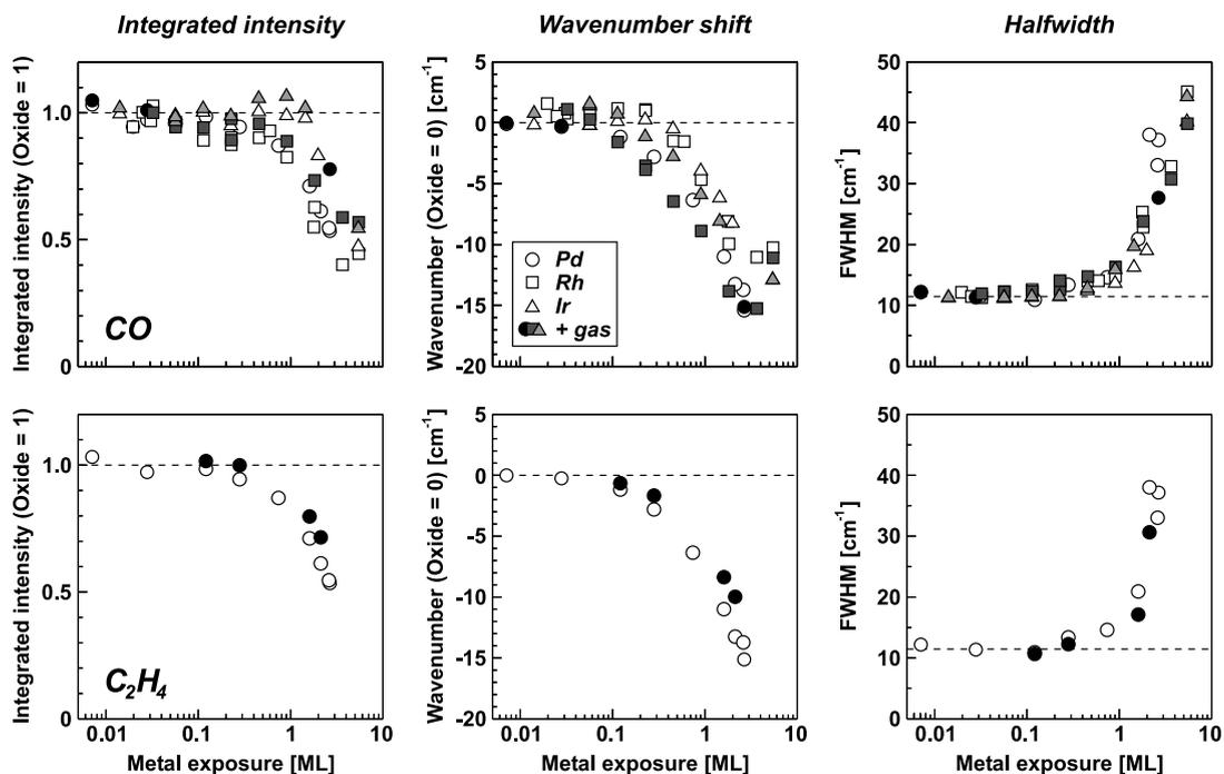
Fig. 6. Integrated intensity relative to the clean oxide film, wavenumber shift relative to the clean oxide film, and halfwidth of the alumina infrared band  $\nu_3$  as a function of metal exposure after metal deposition at 90 K (white symbols) and after gas saturation at the same temperature (shaded symbols). Top: CO adsorption on Pd, Rh, and Ir deposits. Bottom: ethene adsorption on Pd deposits.
