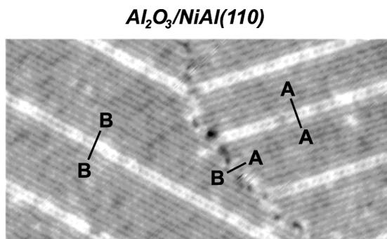
Fig. 1. STM image ( $775\text{ \AA} \times 400\text{ \AA}$ ) of the alumina film grown on NiAl(110). (A–A), (B–B): antiphase domain boundaries, (A–B): reflection domain boundary [31].
