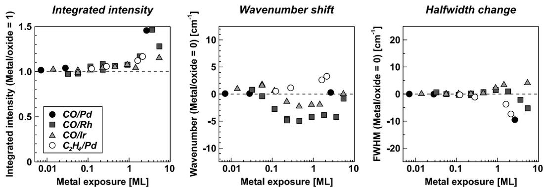
Fig. 7. Gas-induced change in integrated intensity, wavenumber, and halfwidth of the alumina infrared band  $\nu_3$  relative to the metal-modified oxide film as a function of metal exposure. Shaded symbols: CO adsorption on Pd, Rh, and Ir deposits. White symbols: ethene adsorption on Pd deposits.
