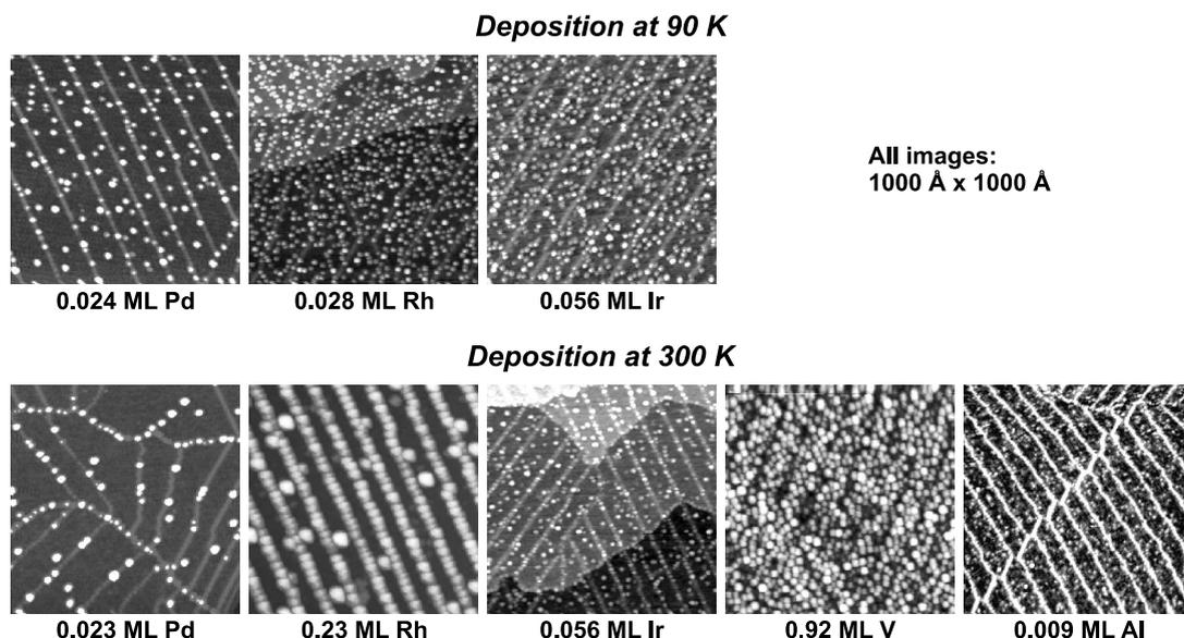
Fig. 3. Room-temperature STM images ( $1000\ \text{\AA} \times 1000\ \text{\AA}$ ) recorded after deposition of submonolayer metal exposures onto the thin alumina film: Pd, Rh, and Ir deposited at 90 K (top) and Pd, Rh, Ir, V, and Al deposited at 300 K (bottom). The line protrusions are domain boundaries of the oxide film.
