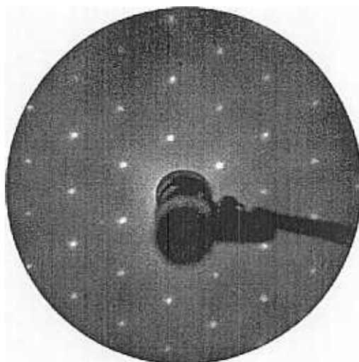
Fig. 16. Low energy electron diffraction diagram of \text{V}_2\text{O}_3(0001) grown on \text{Au}(111) [98]
