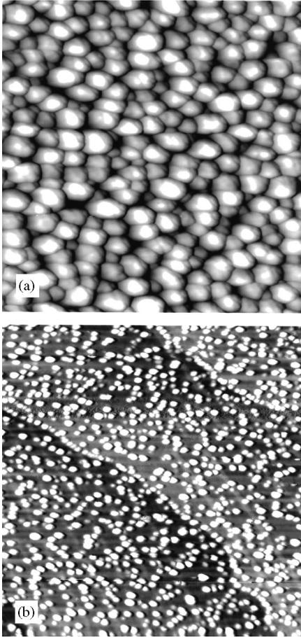
Fig. 1. (a)  $0.3 \text{ \AA}$  Co/ $\text{Al}_2\text{O}_3$ /NiAl(1 1 0),  $200 \times 200 \text{ nm}^2$ / 5.1 V/ 0.5 nA; (b)  $6.5 \text{ \AA}$  Co/ $\text{Al}_2\text{O}_3$ /NiAl(1 1 0),  $100 \times 100 \text{ nm}^2$ / 1.0 V/ 0.56 nA. At both coverages STM shows three-dimensional particles indicating that Volmer–Weber growth mode is present.
