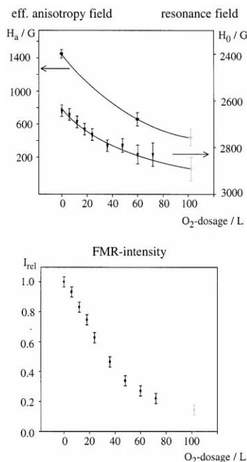
Fig. 3. FMR data of an oxidation series of 6.5 Å Co (annealed) showing increasing tendency towards isotropic SPM: the FMR-intensity decreases with increasing oxygen dosage (lower part); the effective anisotropy field decreases and the resonance field tends towards 3035 G (upper part).
