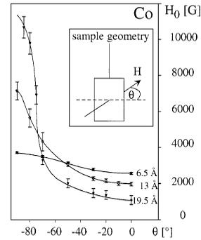
Fig. 2. Resonance field  $H_0$  as a function of the out-of-plane angle  $\theta$  for different amounts of cobalt on sapphire exhibiting a uniaxial out-of-plane anisotropy and an in-plane magnetization.
