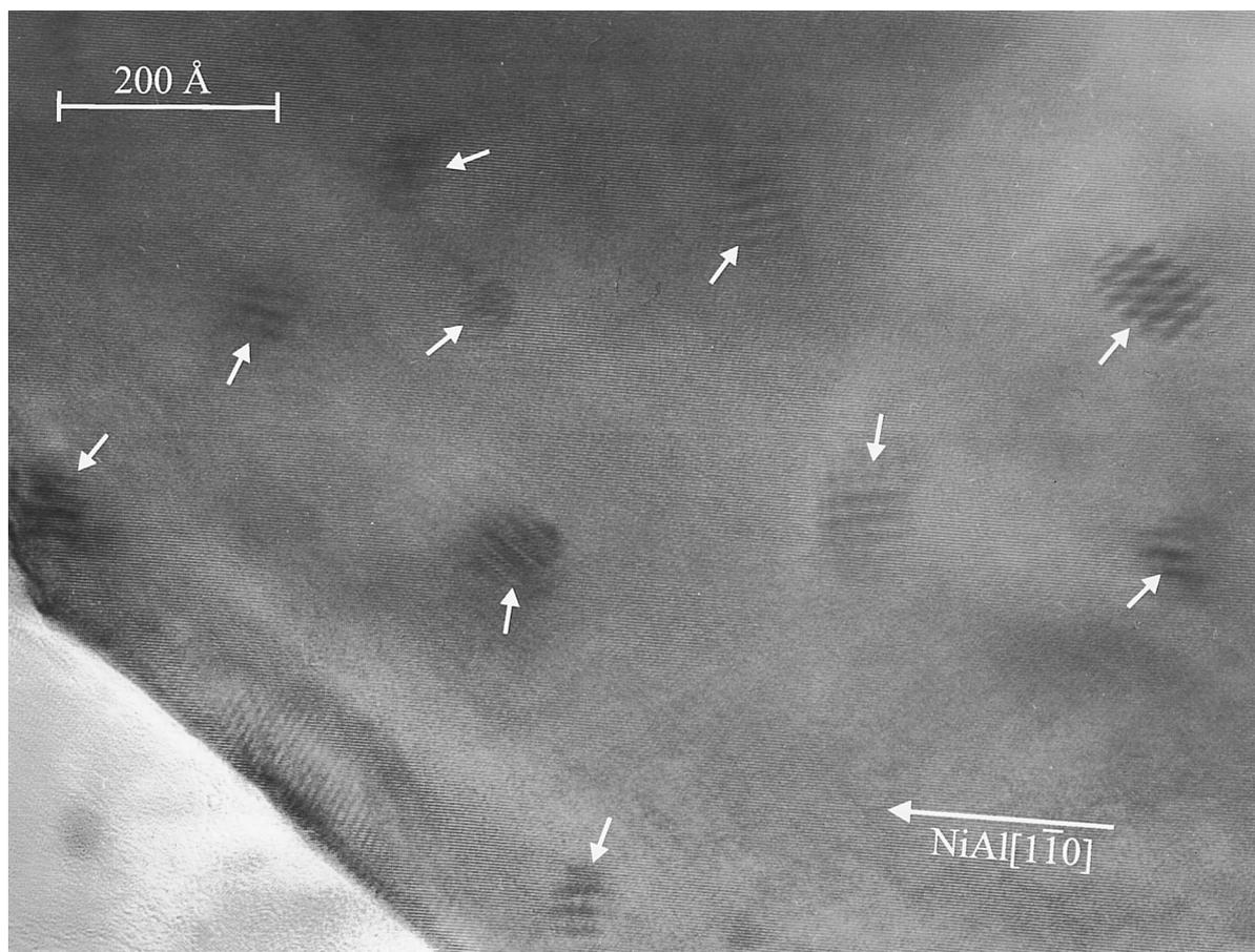
Fig. 3. TEM image of tantalum clusters (see arrows) on  $\text{Al}_2\text{O}_3/\text{NiAl}(110)$ .
