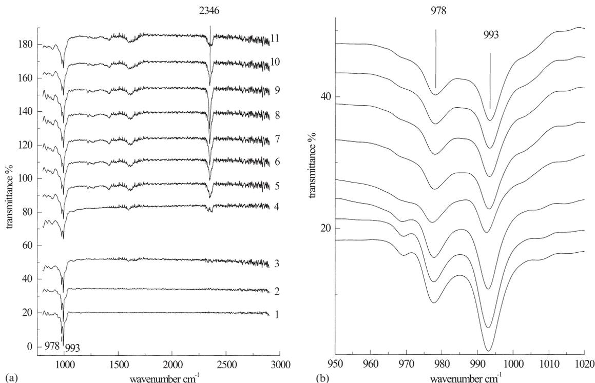
Fig. 11. (a) Infra-red spectra of  $\text{CO}_2$  on oxygen-predosed on polycrystalline  $\alpha\text{-Cr}_2\text{O}_3$  (outgassed at 1073 K). The surface was exposed to 0.1 Torr  $\text{O}_2$  at 100 K (spectrum 1) and subsequently heated up to 300 K (spectrum 3). After recooling to 100 K,  $\text{CO}_2$  (0.1 Torr) was dosed (spectrum 4). In the following, the system was heated stepwise to 300 K again (spectrum 11). (b) Exploded view of the 950–1020  $\text{cm}^{-1}$  interval of (a).
