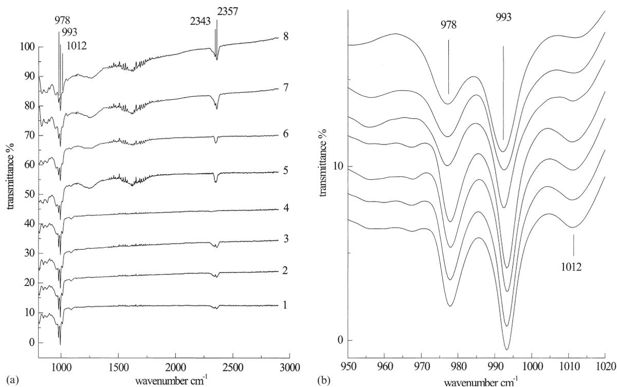
Fig. 10. (a) Infra-red spectra of  $\text{CO}_2$  on oxygen-predosed on polycrystalline  $\alpha\text{-Cr}_2\text{O}_3$  (outgassed at 973 K). The surface was exposed to 0.1 Torr  $\text{O}_2$  at 100 K (spectrum 1) and subsequently heated to 300 K (spectrum 3). After recooling to 100 K  $\text{CO}_2$  (0.1 Torr) was dosed (spectrum 4). In the following, the system was heated stepwise to 300 K again (spectrum 8). (b) Exploded view of the 950–1020  $\text{cm}^{-1}$  interval of (a).
