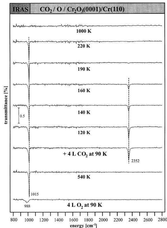
Fig. 7. Infra-red reflection adsorption spectra of  $\text{CO}_2$  on oxygen-pre-dosed  $\text{Cr}_2\text{O}_3(0001)/\text{Cr}(110)$ . The surface was exposed to 4 L  $\text{O}_2$  at 90 K and subsequently flashed to 540 K. After recooling to 90 K, the surface was saturated with  $\text{CO}_2$  (here 4 L dosage). In the following, the system was heated to the specified temperatures.
