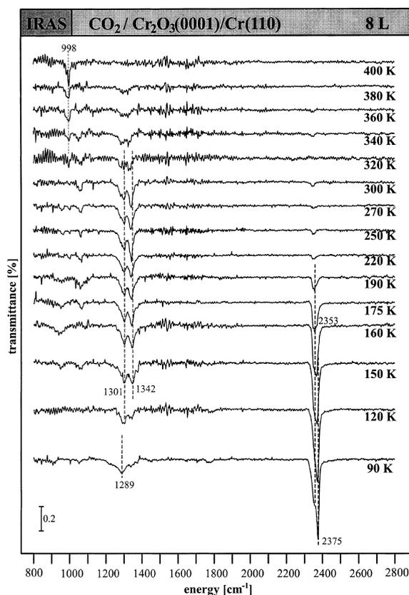
Fig. 3. Infra-red reflection adsorption spectra of  $\text{CO}_2$  adsorbed on  $\text{Cr}_2\text{O}_3(0001)/\text{Cr}(110)$  as a function of temperature after dosing  $8 \text{ L}$  at  $90 \text{ K}$ .
