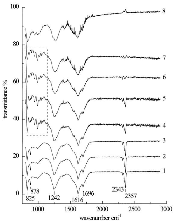
Fig. 9. Infra-red spectra of  $\text{CO}_2$  (0.1 Torr) adsorbed on polycrystalline  $\alpha\text{-Cr}_2\text{O}_3$  (outgassed at 973 K) as a function of temperature. From the bottom, spectrum 1 corresponds to 100 K, and spectra 2–8 are taken at increasing temperatures up to 300 K (spectrum 8).
