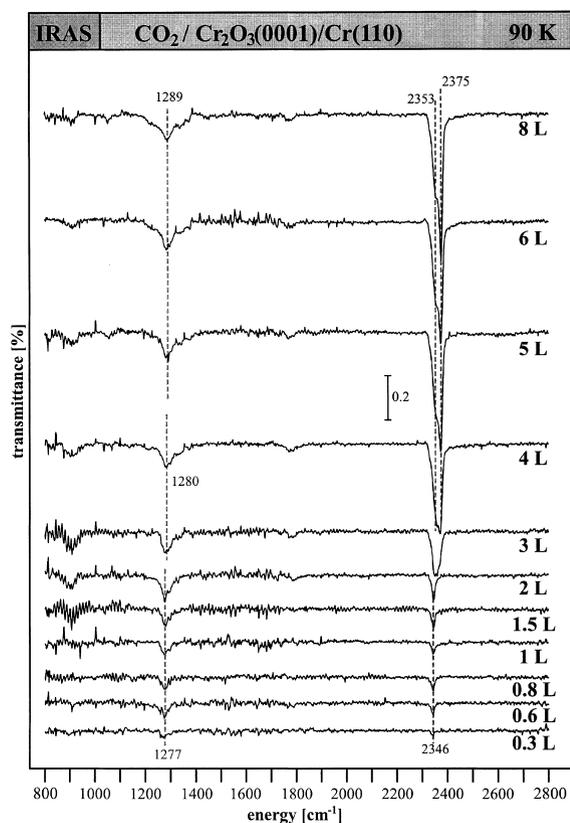
Fig. 2. Infra-red reflection adsorption spectra of  $\text{CO}_2$  adsorbed on  $\text{Cr}_2\text{O}_3(0001)/\text{Cr}(110)$  as a function of dosage.
