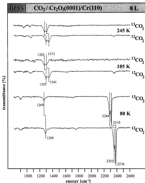
Fig. 4. Comparison of infra-red reflection adsorption spectra of  $^{12}\text{CO}_2$  and  $^{13}\text{CO}_2$  adsorbed on  $\text{Cr}_2\text{O}_3(0001)/\text{Cr}(110)$  as a function of temperature after dosing 8 L at 90 K.
