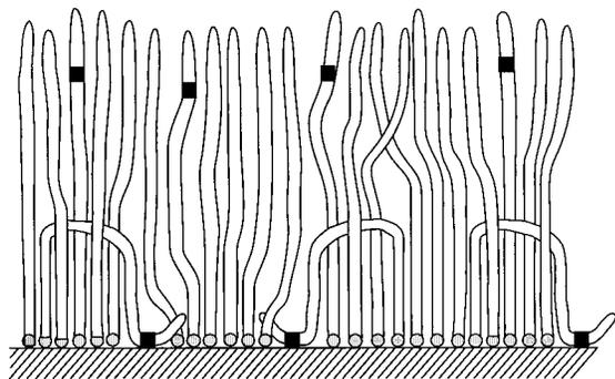
FIG. 12. Schematic representation of loop structures within a 16-doxyl stearic acid film. Squares represents the spin labels, hatched circles the head groups of the molecules.
