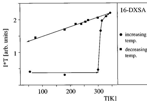
FIG. 11. Curie corrected intensity of a 16-doxyl stearic acid film adsorbed below 25 °C for a temperature cycle from 55 K to 370 K and back to 75 K.
