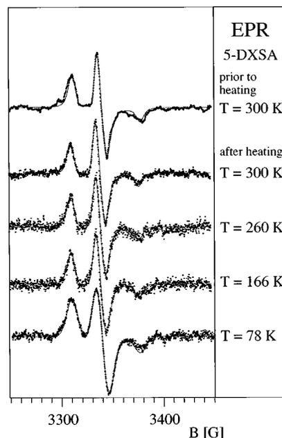
FIG. 2. Temperature dependent EPR spectra of a 5-doxyl stearic acid film after heating to 400 K and then cooling to the given temperature. Points represent the measured spectra, full lines the corresponding simulations. The spectra are normalized to a constant peak-to-peak height.
