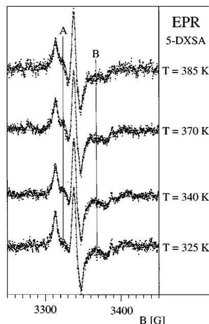
FIG. 8. Temperature dependent EPR spectra of 5-doxyl stearic acid films between 325 and 385 K. Points represent the measured spectra, full lines the corresponding simulations. The spectra are normalized to a constant peak-to-peak height.
