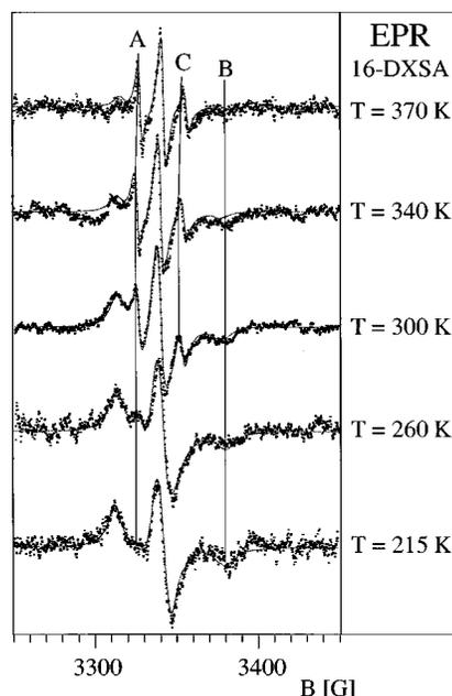
FIG. 3. Temperature dependent EPR spectra of 16-doxyl stearic acid films between 215 and 370 K. Points represent the measured spectra, full lines the corresponding simulations. The spectra are normalized to a constant peak-to-peak height.
