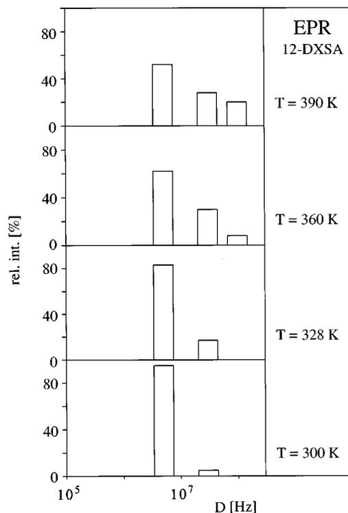
FIG. 7. Relative population of the components used to simulate the spectra of the 12-doxyl stearic acid film shown in Fig. 6.
