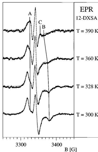
FIG. 6. Temperature dependent EPR spectra of 12-doxyl stearic acid films between 300 and 390 K. Points represent the measured spectra, full lines the corresponding simulations. The spectra are normalized to a constant peak-to-peak height.
