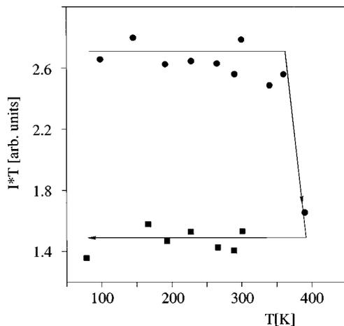
FIG. 1. Curie corrected intensity of a 5-doxyl stearic acid film versus temperature.
