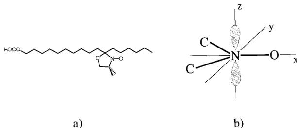
FIG. 4. (a) Schematic representation of a 12-doxyl stearic acid molecule, (b) principal axis of the  $g$ - and  $A$ -tensors for the nitroxides.
