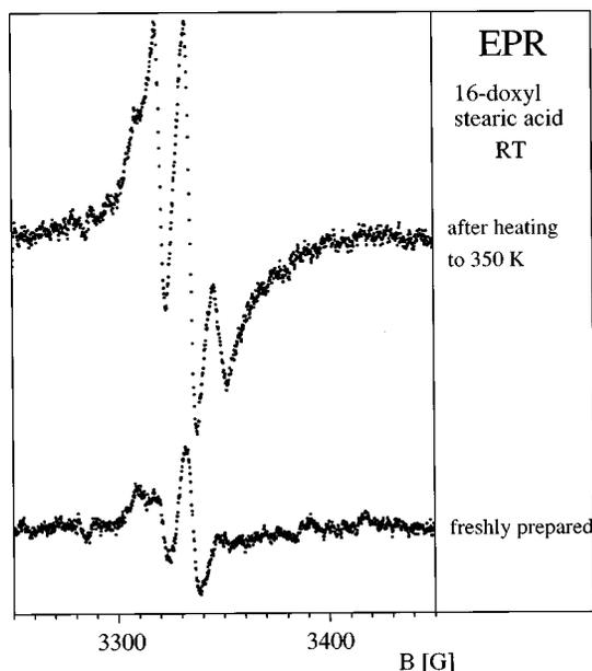
FIG. 10. EPR spectra of a 16-doxyl stearic acid film prepared below 25 °C. Bottom: freshly prepared; top: after heating to 350 K.
