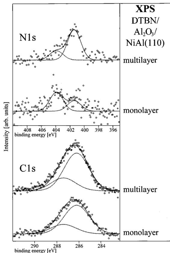
**Figure 3.** XPS spectra from the N 1s and C 1s photoemission of DTBN/ $\text{Al}_2\text{O}_3$ (111). The data are shown in a comparison of multi- and monolayer spectra. The fits are discussed in the text.
