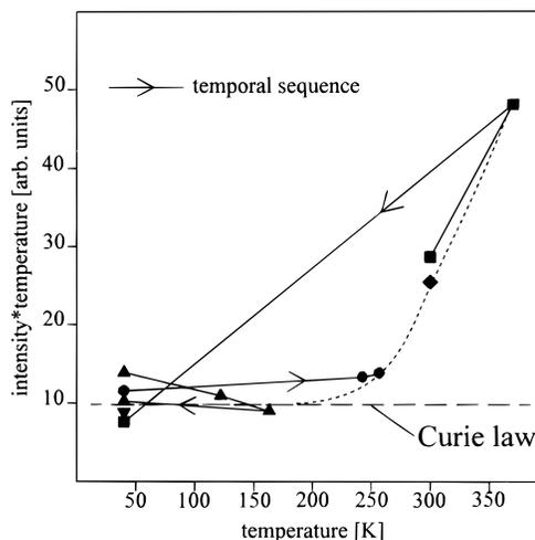
**Figure 7.** Temperature dependence of the integral ESR intensity of monolayer preparations in a Curie-corrected representation. Different symbols represent different preparations. The arrows indicate the sequence of measurements. The dashed horizontal line corresponds to pure Curie paramagnetism.
