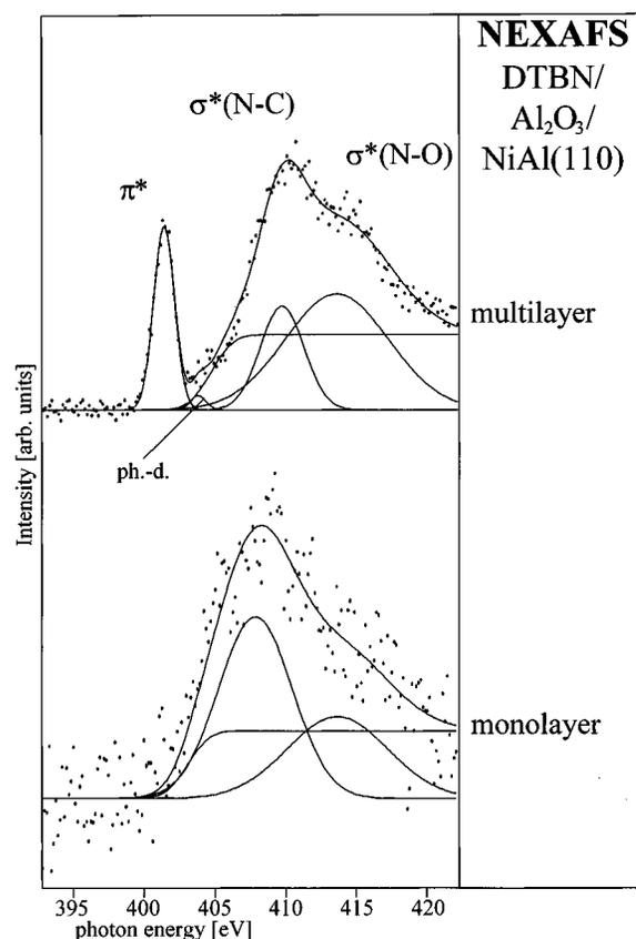
**Figure 4.** NEXAFS spectra from the N edge of DTBN/ $\text{Al}_2\text{O}_3$ (111) in a comparison of multi- and monolayers. The resonances and the fit are described in the text.
