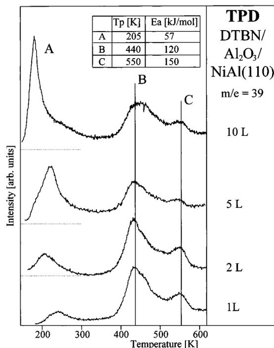
**Figure 2.** Thermal programmed desorption spectra of DTBN/Al<sub>2</sub>O<sub>3</sub>-NiAl(111). The intensity of the fragment with  $m/e = 39$  is shown. One feature from multilayer desorption (A) and two monolayer desorption states (B and C) can be seen. The desorption energies are also given.
