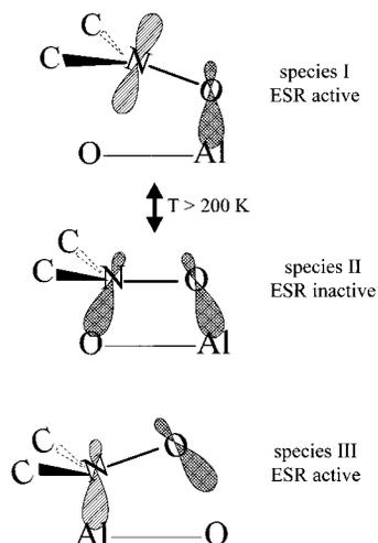
**Figure 10.** Adsorption model for DTBN/ $\text{Al}_2\text{O}_3(111)$ . The three adsorption species discussed in the text are illustrated. The exchange between species I and II is indicated. The Al–O distance in the surface corresponds to the sum of the ionic radii.
