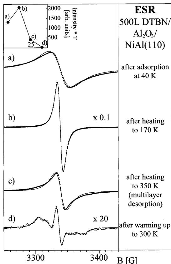
**Figure 5.** ESR spectra of DTBN/Al<sub>2</sub>O<sub>3</sub>(111). The changes going from multi- to monolayer coverages (a–c) are shown. The effect of an equilibrium in the monolayer (c, d) is also presented. The inset displays the course of the integral intensities of the spectra.
