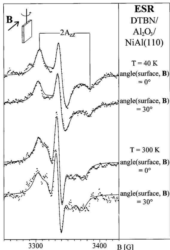
**Figure 6.** Angular dependence of the monolayer ESR spectra of DTBN/ $\text{Al}_2\text{O}_3$ (111). The experiment was done at 40 (two uppermost spectra) and 300 K (two lowermost spectra). The sketch illustrates the turning angle.
