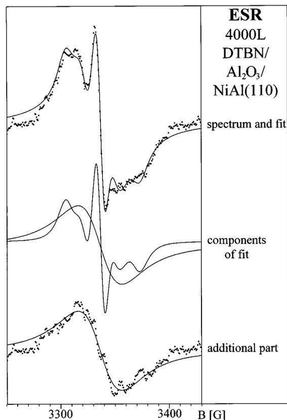
**Figure 8.** ESR spectrum of DTBN/Al<sub>2</sub>O<sub>3</sub>(111) adsorbed at room temperature (top). A decomposition of the simulation (middle) as well as the separated additional part in the spectrum (bottom) is also shown.
