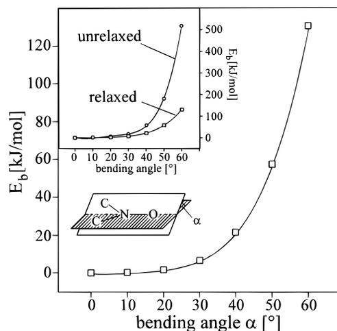
**Figure 11.** Effects of a bending of the molecular frame on the internal energy of the DTBN molecule obtained from ab initio calculations. The sketch illustrates the bending angle  $\alpha$ . The inset shows the influence of relaxation on the molecule's other structural parameter. See text for further explanation.
