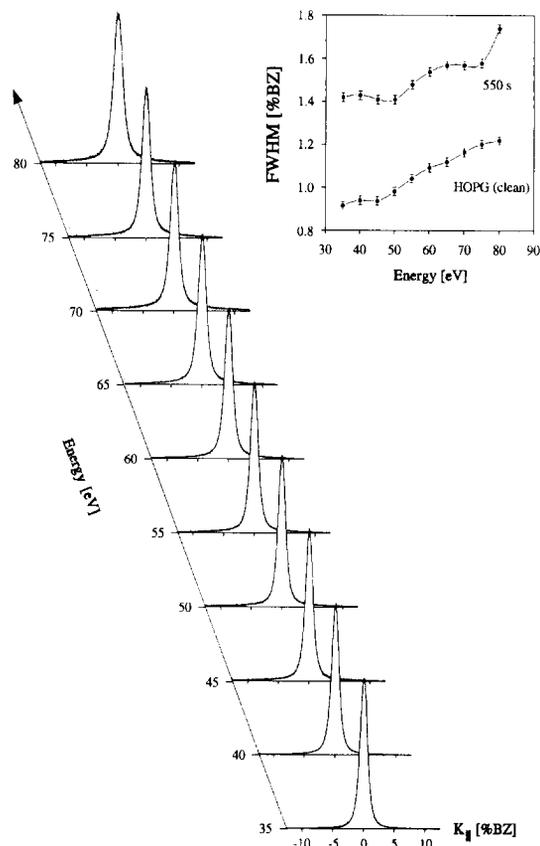
Fig. 6. Energy series of the LEED spot profiles obtained after deposition of Ni at room temperature (550 s). Inset: full width at half maximum of the profiles as a function of energy before and after deposition. The monotonous increase of the halfwidths in both cases is owing to the mosaic structure of the substrate. The additional oscillations have been identified as instrumental artifacts in the case of the clean substrate.
