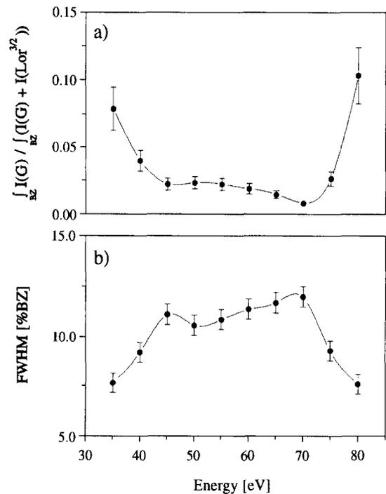
Fig. 4. Integrated intensity of central peak in relation to the total spot intensity (a) and full width at half maximum of the  $\text{Lor}^{3/2}$  shoulder (b) at different energies (deposition time: 550 s).
