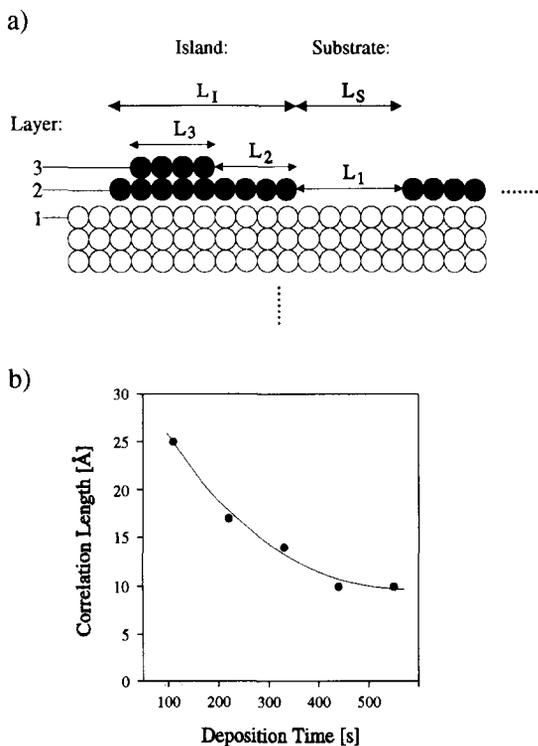
Fig. 5. (a) Definition of terrace lengths for three-dimensional heteroepitaxial islands. (b) Plot of the correlation lengths  $L$  as calculated from the FWHM of the  $Lor^{3/2}$  shoulder at 35 and 80 eV (see Table 1).  $L$  results from  $\bar{L}_1$  and  $\bar{L}_s$  as given by Eq. (1).
