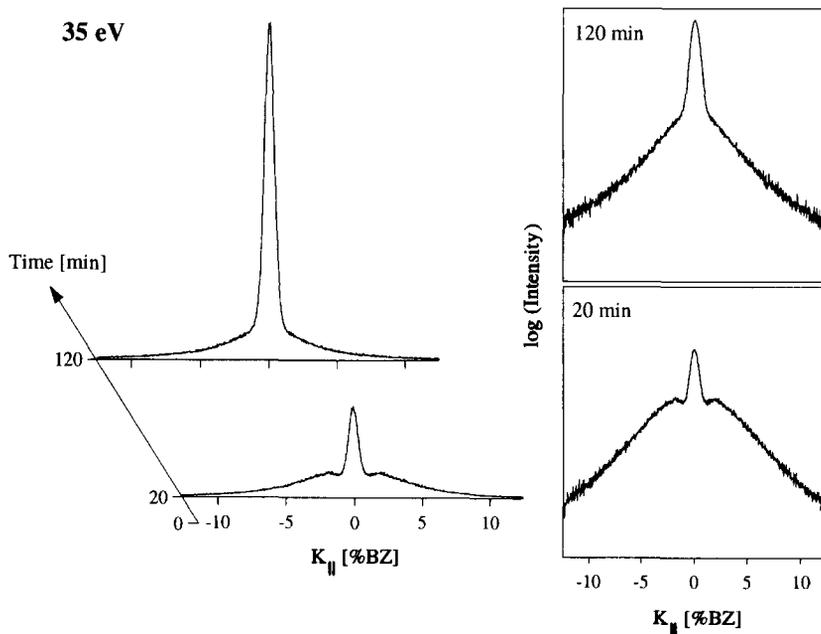
Fig. 2. Profiles of the (00) LEED spot for an electron energy of 35 eV as a function of time after depositing Ni for 550 s at 90 K. A similar development of the spot profiles at that energy was observed for shorter deposition times as well. The parallel component of the scattering vector on the X-axis is given in percent of the Brillouin zone of graphite.
