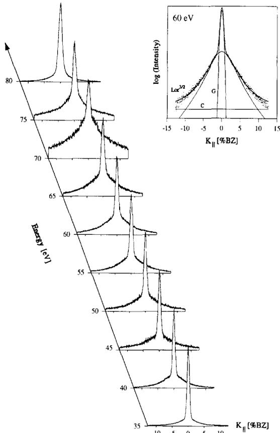
Fig. 3. Spot profiles as a function of energy for the deposition at low temperature (550 s). The profiles have been recorded approximately two hours after the evaporation. The inset shows a representative least-squares fit of the profile at 60 eV (G: Gaussian function,  $\text{Lor}^{3/2}$ : modified Lorentzian function, C: constant background).
