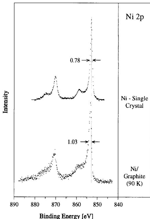
Fig. 7. Comparison between the Ni 2p spectra of a Ni(111) single crystal and Ni deposited on graphite (330 s, 90 K). The first spectrum was recorded with a transmission energy of 25 eV, the second with a transmission energy of 50 eV (loss of resolution by a factor of 1.2).
