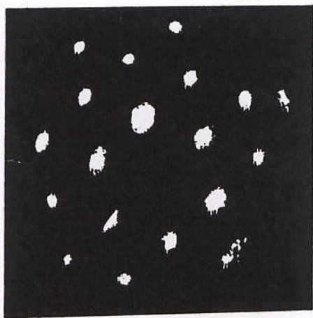
Fig.1a: LEED pattern of \text{Cr}_2\text{O}_3(111)
